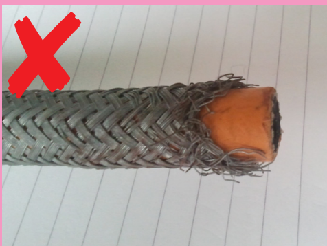
The braided hose is frayed.
